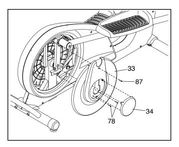
Then, remove the M4 x 15mm Machine Screw (87) and the two M4 x 16mm Screws (78) from the right Disc (33), and then remove the right Disc.
