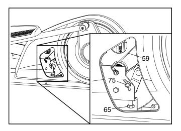
When the Drive Belt (59) is tight, tighten the Idler Screw (75). Then, reattach Access Cover (29) and plug in the power adapter.
