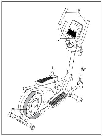
Push the pedals (L) until they begin to move with a continuous motion. Note: The pedal discs (M) can turn in either direction. It is recommended that you move the pedal discs in the direction shown by the arrow; however, for variety, you can turn the pedal discs in the opposite direction.
