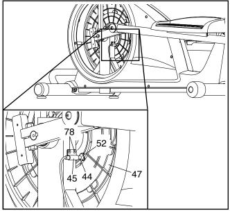
Next, rotate the Pulley (47) until a Magnet (52) is aligned with the Reed Switch (44). Slide the Reed Switch slightly toward or away from the Magnet. Then, retighten the M4 x 16mm Screws (78).
