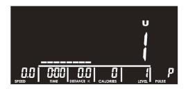
Use the arrow buttons UP and DOWN to select the user program "U". Use the arrow buttons UP and DOWN to prepare a USER program. Using the arrow buttons, enter the resistance level for each segment and press ENTER to confirm. When complete, press and hold ENTER for two seconds to move to the time selection. After entering your desired workout time, start your workout by pressing the START/STOP button.
