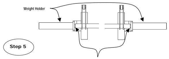
Step 5: Adjust the spacing between the Weight Holders and the ends of the Red Weight Bar Assembly by moving the Linear Bearing Shafts in or out (using the adjustment slots in the Top and Bottom Shaft Mounts) before final tightening of the bolts. These components should not rub or bind when working out.
