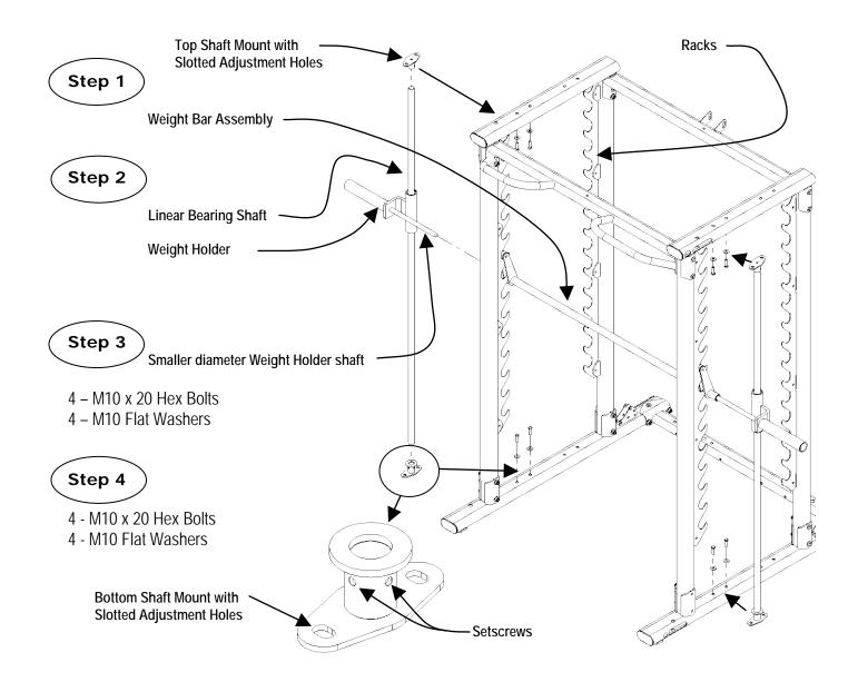
Step 1: Position the Red Weight Bar Assembly on the Hooks of the front Racks.
