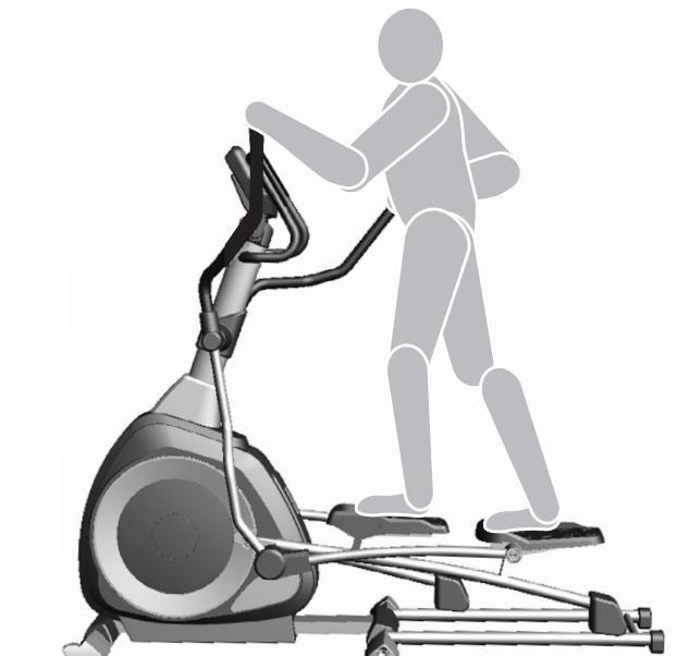
Make sure you are standing firmly and securely on the footboards. The sole of the shoe may meet the front end of the footboard (especially with small people).
