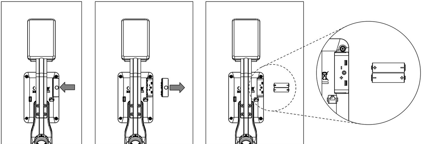
A weak or an extinguished computer display makes a battery change necessary. The computer is equipped with two batteries. Perform the battery change as described below:
