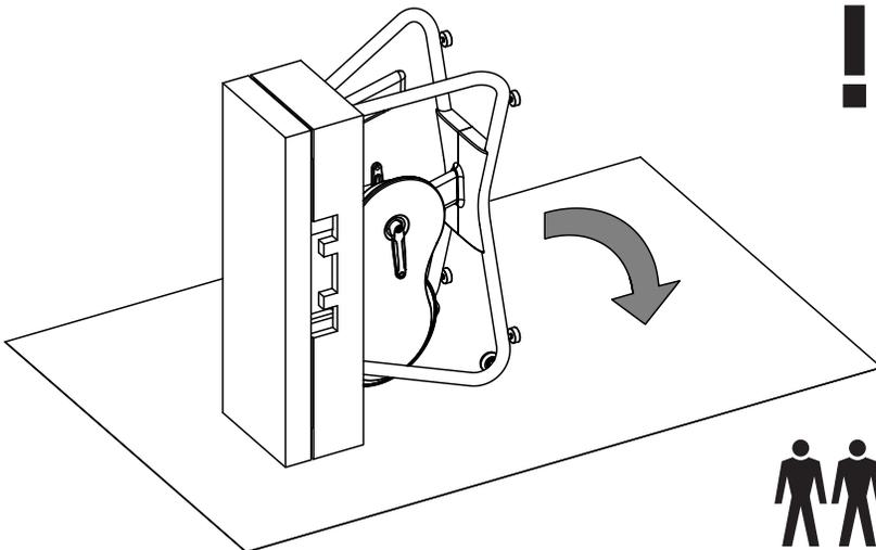
**EN** **WARNING!** Note that the HOI FRAME bike is very heavy and care must be taken as the bike is rotated from upside down position to the upright position. It is highly recommended that two adults perform this operation. The bike and packaging must be supported together during this process.
